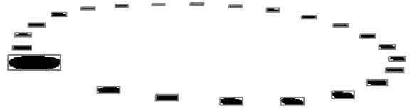
Figure 2. Boxes enclosing calibration pattern dots (colors inverted for ease of viewing)
